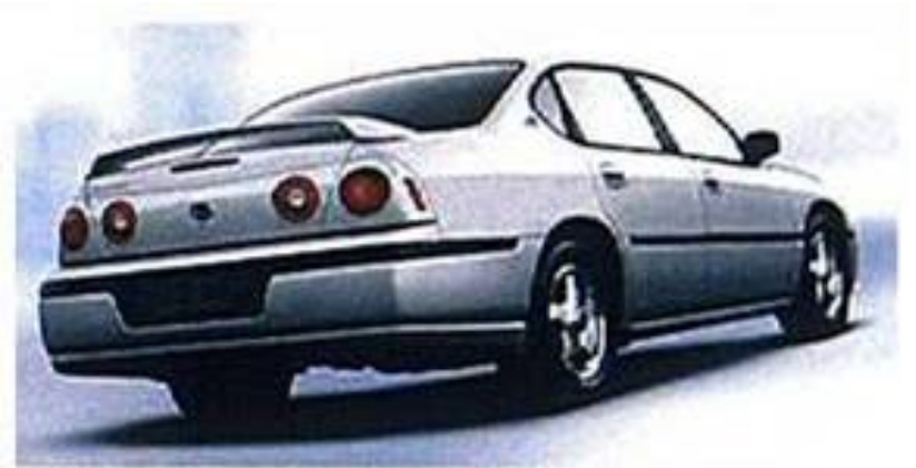
245 tonnes / year of nanocomposites. Polypropylene side body mouldings reinforced with montmorillonite
